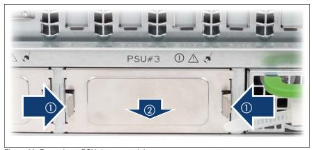
Figure 20: Removing a PSU dummy module
